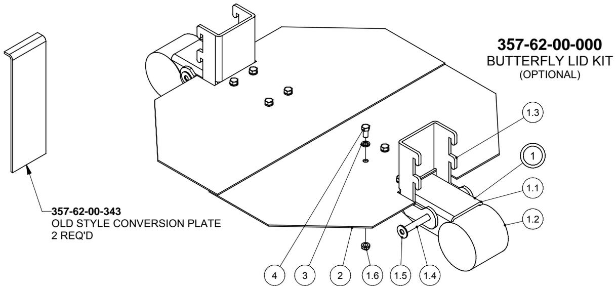
NOTE: WITH INSTALLATION OF A BUTTERFLY LID, A SAFETY GRATE MUST BE USED TO LOCK LID IN PLACE
